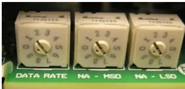
Figure 2-A Rotary Switches – Manual Setup
